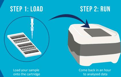
**AUTOMATED WESTERN BLOTS** utilize microfluidic or capillary cartridges to analyze relative protein size and abundance, minimizing setup, sample volume, time to results, and reagent waste
